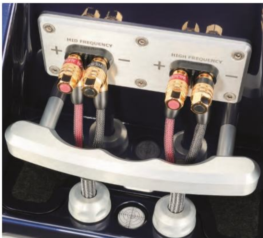
ABOVE: Cables from the main crossover pass up through the top of the Puppy, behind the WATT's alloy rear handle, and terminated in gold-plated 4mm/spade posts. The WATT's height is adjustable at the rear, pivoting on two fixed front spikes for fine adjustment of overall time alignment
